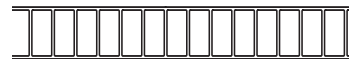
BRICK HEADER BRICK SIZE: 3 \frac{7}{8}'' \times 7 \frac{5}{8}'' ROLL WIDTH: 8 \frac{3}{4}'' JOINT WIDTH: \frac{1}{2}''
