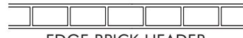
EDGE BRICK HEADER BRICK SIZE: 4 \frac{1}{8}'' \times 8 \frac{15}{16}'' ROLL WIDTH: 5 \frac{1}{8}'' JOINT WIDTH: \frac{1}{2}''
