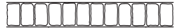
COBBLE HEADER BRICK SIZE: 4 \frac{3}{4}'' \times 7 \frac{1}{2}'' ROLL WIDTH: 8 \frac{5}{8}'' JOINT WIDTH: \frac{1}{2}''
